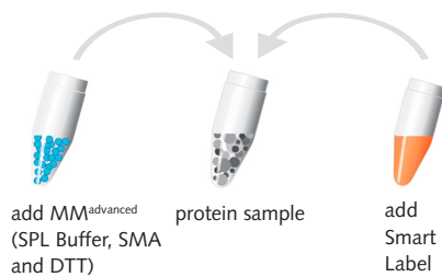
Fig. 1. Sample preparation for total protein SPL labeling incl. SMAs.
